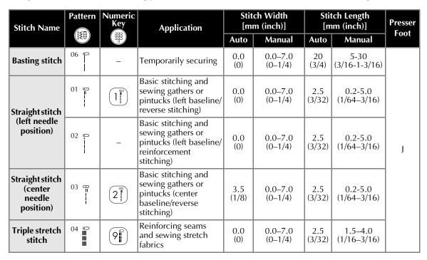
Straight stitches are used for sewing plain seams. Five stitches are available for basic stitching.
