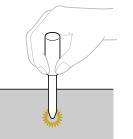
• When using the eyelet punch, place thick paper or some other protective sheet under the fabric before punching the hole in the fabric.
