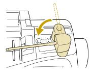
Place the upper thread spool for the needle on the right side onto the extra spool pin, and then secure it with the spool cap.
