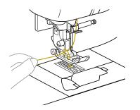
**5** Pull out about 10-15 cm (4-5 inches) of the bobbin thread under the presser foot toward the rear of the machine.
