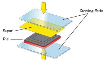
1. Place an Originals or Bigz Die on a Cutting Pad with foam side up. Place paper or desired material to be cut on top of the die. Place the second Cutting Pad on top of the paper or material to create a "sandwich."
