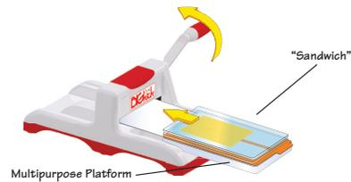
2. Place sandwich on Multipurpose Platform and slide Platform into opening of BIGkick. Note the rotation of the handle and continue to rotate it in the same direction until the Platform has passed through the opening and the rollers. Remove Platform from BIGkick. Your die-cut shape is ready to use!
