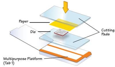
1. Place Sizzlits Die onto a Cutting Pad with foam side up. Place paper over the die. Place another Cutting Pad over the paper to create a "sandwich." For Clearlits Die, place die over photo or material so that the area to be cut shows through the die. Then place photo or material and die between Cutting Pads to make sandwich.
