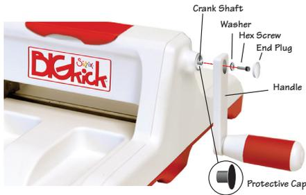
Before attaching handle, remove protective cap on crank shaft and discard. Then attach handle by sliding washer over hex screw and insert through handle and into crank shaft. Tighten hex screw with hex wrench provided with handle kit. Press end plug over hex screw until firmly sealed.
