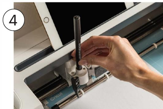
Insert Infusible Ink Pen or Marker into Clamp A, load mat into machine, then press flashing **Go** button. **Tip:** If you have assigned multiple pen colors to your design, Design Space will prompt you to load specific colors at specific times.
