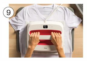
Press at 385°F for 40 seconds. Press the green C button to start the timer countdown.
