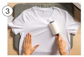
**Do not skip this step:** Use a fresh adhesive to lint roll the entire surface. Even small debris or fibers can cause imperfections in the final transfer.
