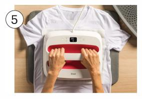
**Do not skip this step:** Preheat application area to remove moisture and wrinkles to avoid unwanted effects. For this project, press at 385°F for 15 seconds. Remove butcher paper and let item cool completely.
