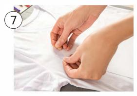
Tape down each corner of the design with heat resistant tape. This keeps your design from shifting during transfer.
