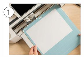
Place sheet of copy paper onto a LightGrip Machine Mat.
