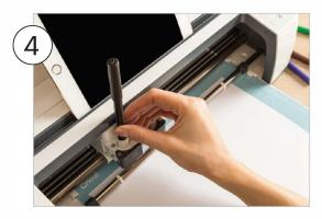
Insert Infusible Ink Pen or Marker into Clamp A, load mat into machine, then press flashing **Go** button.
