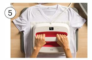
**Do not skip this step:** Preheat application area to remove moisture and wrinkles to avoid unwanted effects. For this project, press at 385° F for 15 seconds. Remove butcher paper and let item cool completely.
